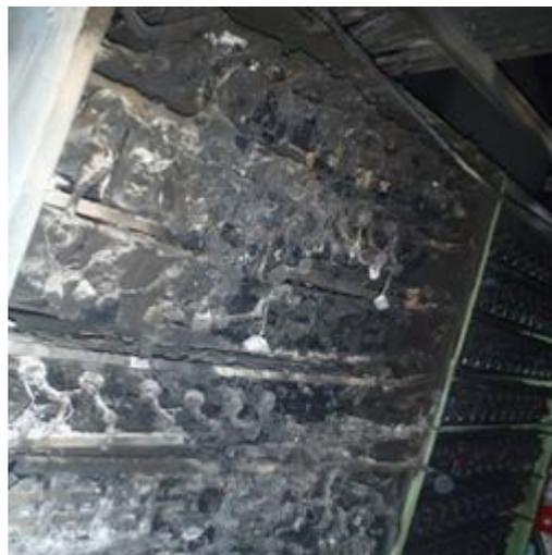
**Figure 2 – Battery cabinet with doors removed. Damage within left cabinet.**
